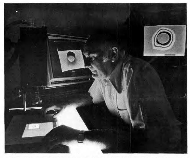
BILL MOTTERN (9351) demonstrates new image analyzer system in Nondestructive Testing laboratory. Photographic image of test item can be manipulated through a TV camera, a mini-mini computer, a three-dimensional graphics screen and a color TV monitor to gain desired information.
